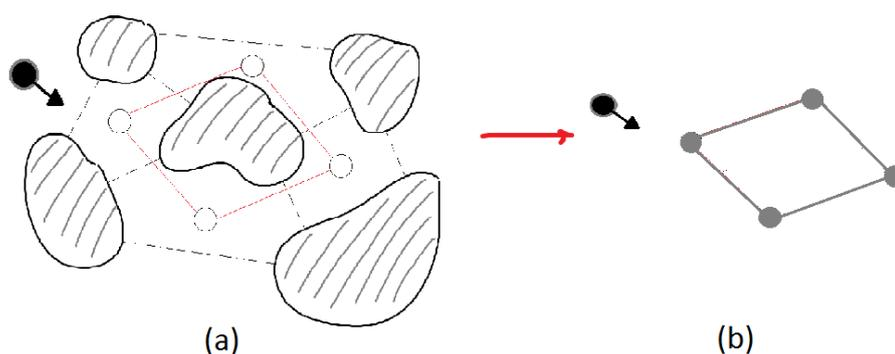
Figure 15: Diffusion of a particle in a porous medium (a) is modeled by a continuous time random walk on a porous graph (b).
