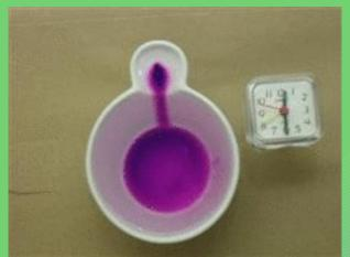
Dominating effect: density-driven flow Diffuse concentration profiles, no "interference"
