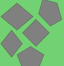
Delayed hydration poor use of clinker **Dissolution of unreacted** cement clinker increasingly impeded by CSH diffusion barrier
