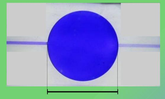
Washing out a blue colour tracer (C.I. Basic Violet 3) from a circular flat cell
