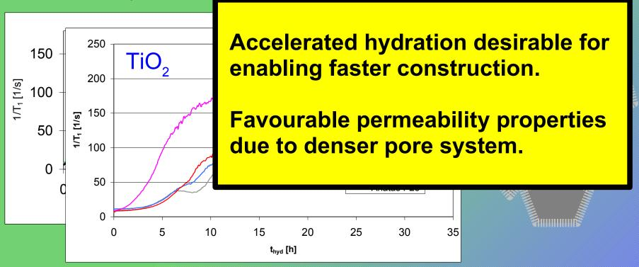
Cement hydration kinetics studied by TD-NMR 1/T<sub>1</sub> essentially proportional to S/V inside cement stone matrix
