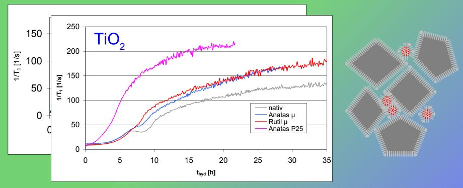
Cement hydration kinetics studied by TD-NMR 1/T<sub>1</sub> essentially proportional to S/V inside cement stone matrix
