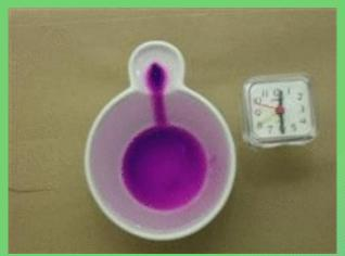
Dominating effect: density-driven flow Convection cells, "interference"
