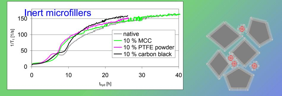
Cement hydration kinetics studied by TD-NMR 1/T<sub>1</sub> essentially proportional to S/V inside cement stone matrix
