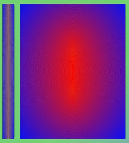
Substantially higher temperatures in extended objects (e.g. over 80 °C in massive concrete structures vs. almost neglegible heating in slender structures)
