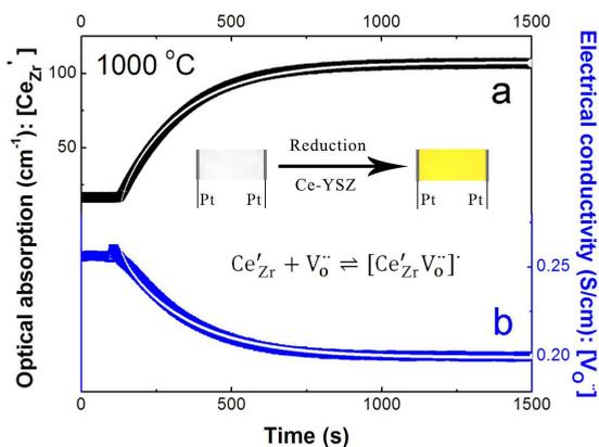
Figure 1: Relaxation experiments on  $Ce_{0.08}Y_{0.2}Zr_{0.72}O_{1.9}$  upon  $a_{O_2}$ -jump from  $O_2$  to  $ArH_2$  at  $1000\text{ }^\circ\text{C}$ , (a) optical absorption and (b) electrical conductivity, monitored by optical spectroscopy and electrochemical impedance spectroscopy under in-situ conditions, respectively, showing the evidence for defect interactions in Ce-YSZ upon reduction. The white solid lines are fits to a kinetic model involving  $k_{chem}$  and  $D_{chem}$ .
