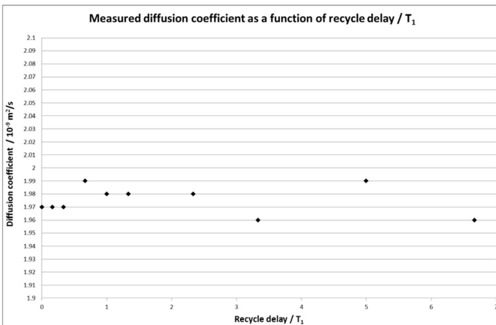
Figure 4.5 Varying the recycle delay on a doped water sample ( $T_1 \sim 300$  ms) using the spoiler recovery 13-interval PFGSTE.
