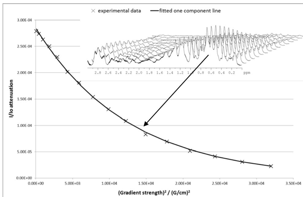
**Figure 4.6** The spoiler recovery 13-interval PFGSTE applied on lysozyme sample.
