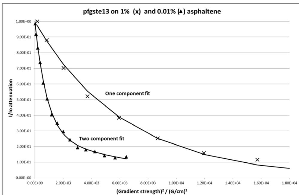
Figure 4.7 The spoiler recovery 13-interval PFGSTE applied on asphaltene samples
