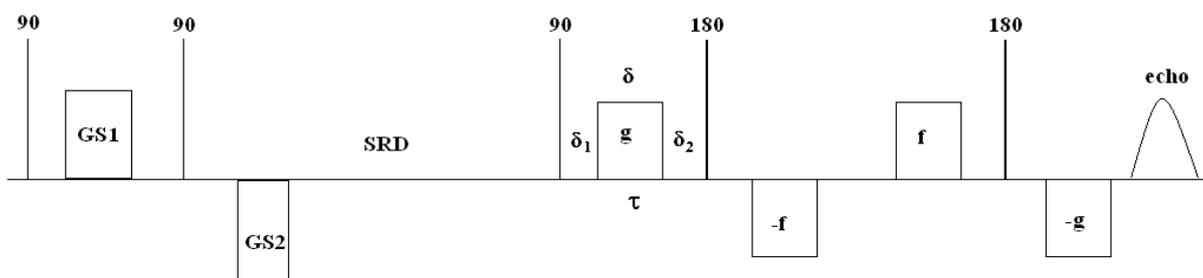
**Figure 4.1** The combined spoiler recovery 11-interval PFGSE sequence
