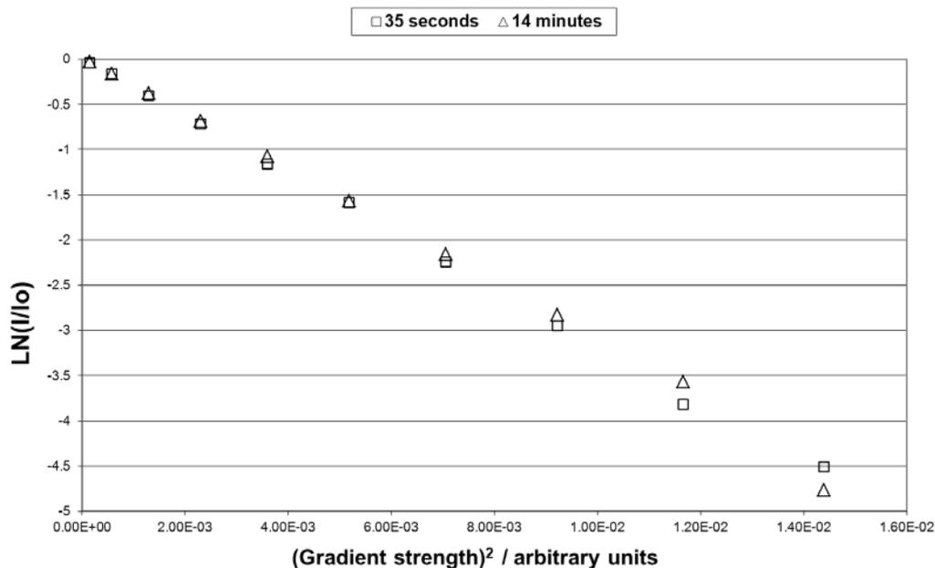
**Figure 4.2** Comparison of the 11-interval PFGSE with the spoiler recovery (total experimental time of 35 seconds) and without the spoiler recovery (total experimental time of 14 minutes) on pure water.
